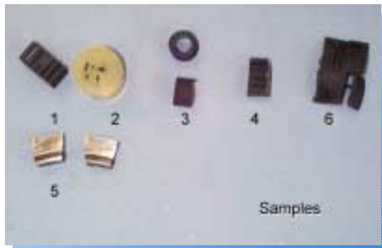
Figure 1: Image showing the various samples cut using the Model 660 Low Speed Diamond Wheel Saw. Materials ranging from rubber, metal rubber composites, encapsulated samples, and metals were all cut using the Model 660.
